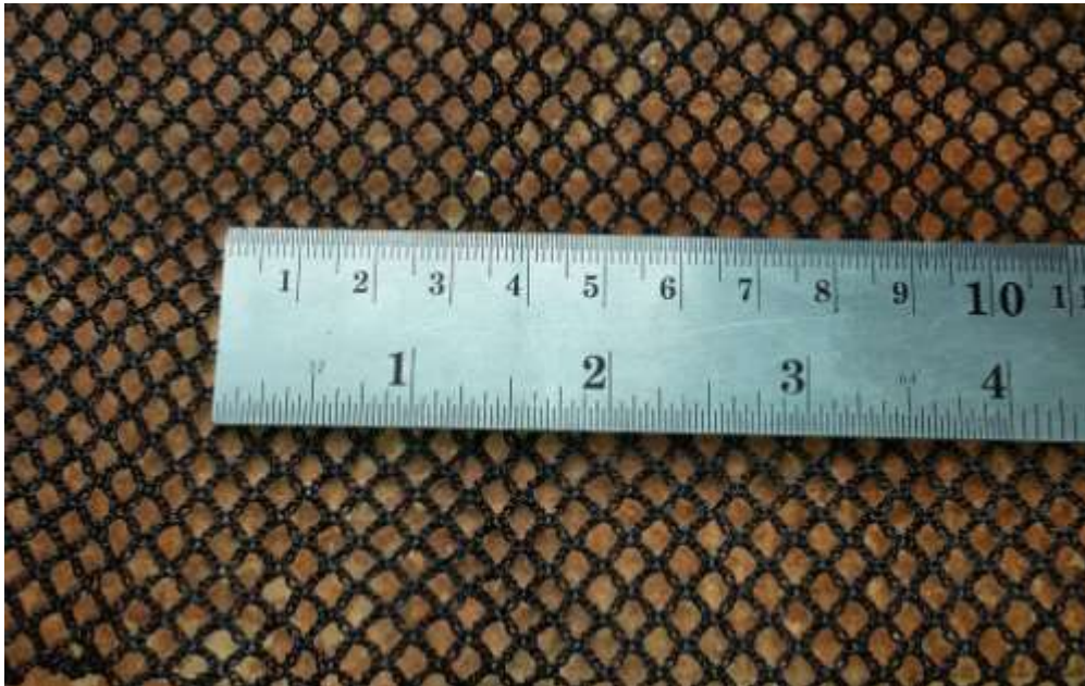
Fish net Kap 8 mm, 50m x 3 m rolls, 153 gram/m 2
